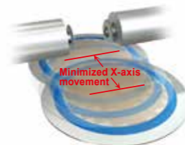
TWIN Dicing concept with the face-to-face twin-spindles
