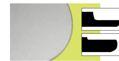
Terrace Grinding Counter Measure against Knife Edge/Asymmetric Profile Grinding
