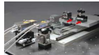
Slim Type 3-axis Measuring Interferometer
