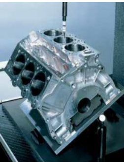
Measurement example of cylinder block and crankshaft.
