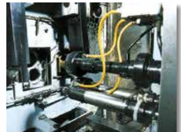
Internal diameter measuring system for lathe post-process
