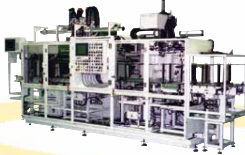
Cylinder block measuring and marking machine Automated machine that measures bore diameters for crankshaft, as well as crankshaft bore coaxiality, and marks a prescribed position.
