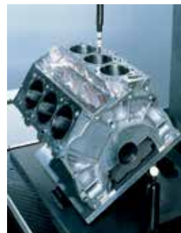
Measurement example of cylinder block and crankshaft.
