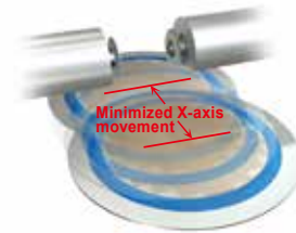
TWIN Dicing concept with the face-to-face twin-spindles
