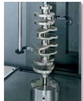
Measurement example of cylinder block and crankshaft.
