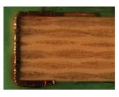
Electrode cutting UV-TAPE (PO TYPE) 18,000 1/min<sup>-1</sup> 50mm/sec
