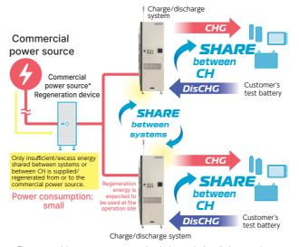
\* The commercial power source regeneration device can be installed separately within the system in the same way as our conventional systems
